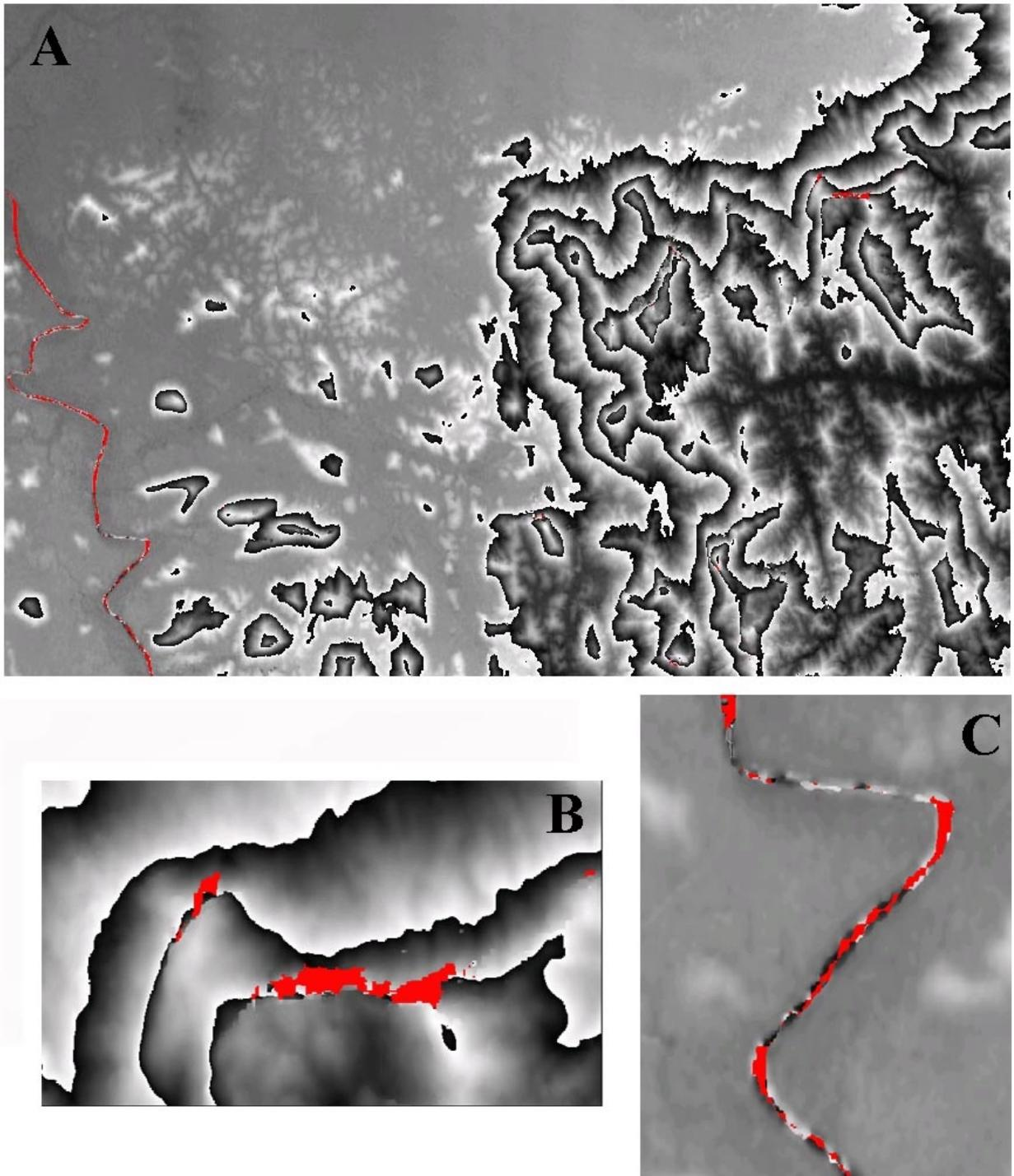
**Image 2:** Gaps detected in map sheet 7021ii: A: Full map; B: Detail of gaps associated to high slopes; C: Detail of gaps associated to water bodies.
