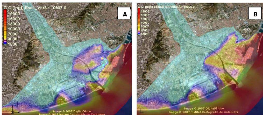
*Forecast of chloride concentration in the Llobregat Delta aquifer for the year 2036. (A) With hydraulic barrier (B) Without hydraulic barrier nor infiltration ponds. Source: Ortuño, 2009.*
