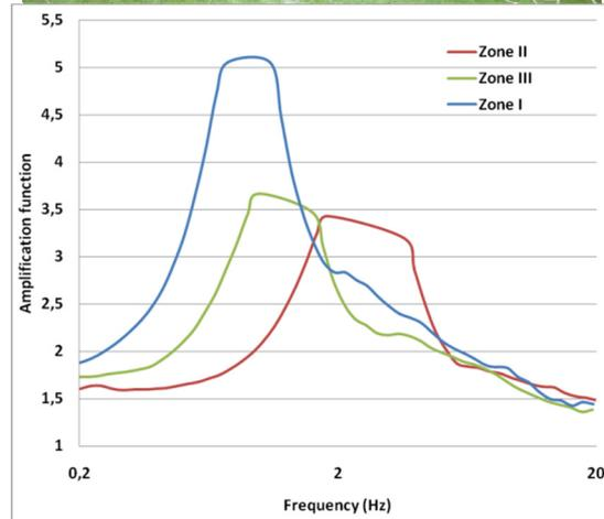
Top: Pictures during the geophysical survey in the Camp Nou Stadium. Bottom: H/V seismic noise spectral ratio and amplification function for the three zones identified in the seismic microzonation studies performed in Barcelona city.
