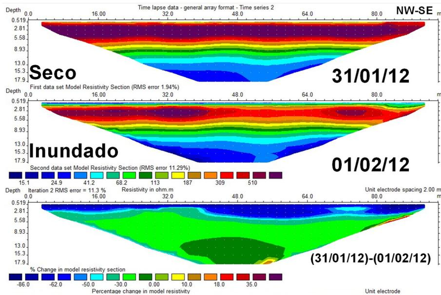
*Geoelectrical sections. Up: dry pond. Center: inundated pond. Down: porcentual variation of electrical resistivity between the dry and flooded models (Sendrós, 2016).*
